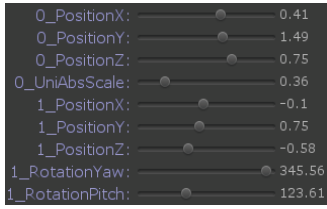
Figure 5. A design vector for a scene with two cubes. The first cube can be positioned and scaled uniformly. The second cube can be positioned and rotated around the X and Y axis. This defines the design space of this scene for the optimization algorithm.
