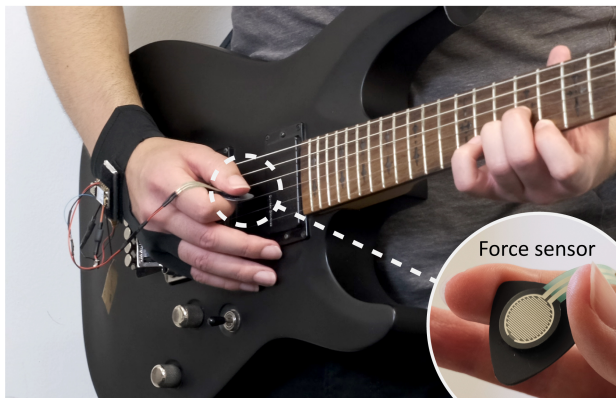
Figure 1: We present PressurePick, a wearable device that unobtrusively records pressure on a guitar pick in order to estimate muscle tension. a) First, the learner uses our PressurePick device while practicing a song. b) Based on the recorded pressure time series of the guitar pick, we estimate the learner’s muscle tension. Our front end visualizes the estimated muscle tension for the whole song and for each part. In the UI, the learner can click on a part for detailed inspection.
