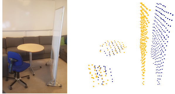
Figure 9. During our evaluation, participants did not arrange the furniture exactly in the same way after recreating layouts repeatedly. This example shows a state with a table, a chair and a whiteboard. The participant unknowingly put the whiteboard about 30 centimeters away (orange) from where it was captured (blue). SpaceState still successfully identifies the state, also while people move within it.
